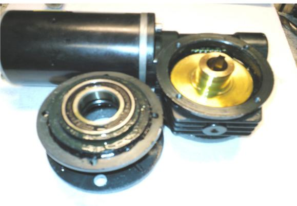
Fill with gear oil EP90 or simmilar. Fill up just over the brass chrown wheel.
